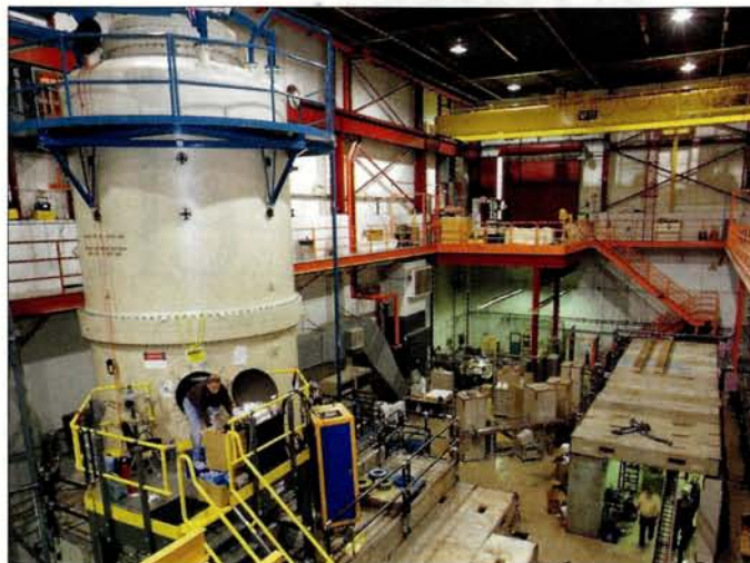
Left: the world's first electron-cooling device installed in the NAP-M ring at Novosibirsk in the early 1970s. Right: Fermilab's electron-cooling project facility is based on a Pelletron accelerator (left), which produces a continuous high-current electron beam. An 18 m cooling section is under construction (right). (Fermilab Visual Media Services.)
