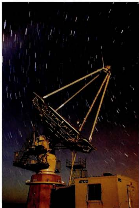
The 10 m CANGAROO II air Cerenkov telescope in Woomera, South Australia, is tracing the origins of cosmic rays. (CANGAROO.)
