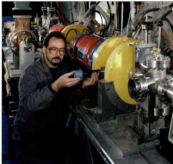
At work on the drive line of the Argonne Wakefield Accelerator Facility. The witness line can be seen in the background.
